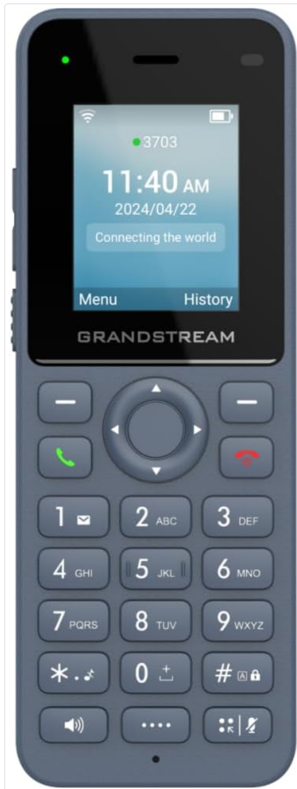
Figure 1: Front view of the Grandstream WP816 Wi-Fi Phone, displaying its screen, keypad, and branding.
