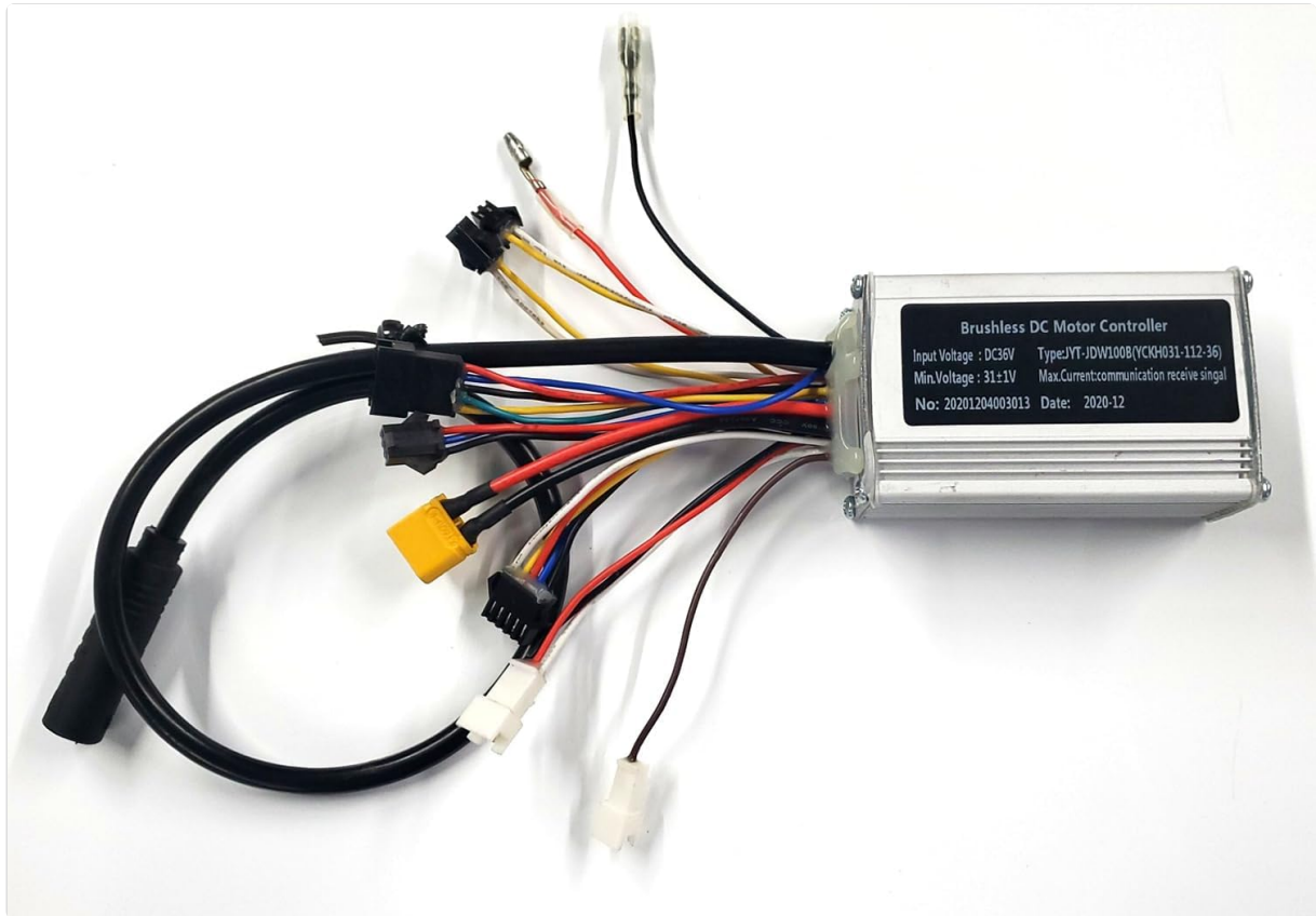
Image 1: Swagtron EB7 / EB-7 Plus eBike Brushless DC Motor Controller. The image displays the silver controller unit with numerous colored wires and connectors, including an Xt60 quick disconnect, extending from its side. A label on the controller shows "Brushless DC Motor Controller," "Input Voltage: DC36V," "Min.Voltage: 31±1V," and other technical specifications.
