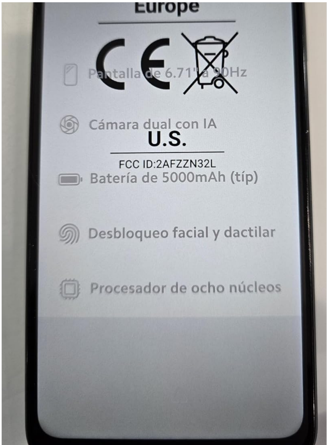
Figure 3.2: Redmi A3X Certification Information. This image shows the phone's screen displaying regulatory details such as the model number (24044RN32L), FCC ID (2AFZZN32L), and battery capacity (5000mAh).
