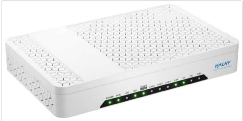
Figure 4.1: Front view of the Halny HL-4GXV-F GPON ONU with LED indicators.
