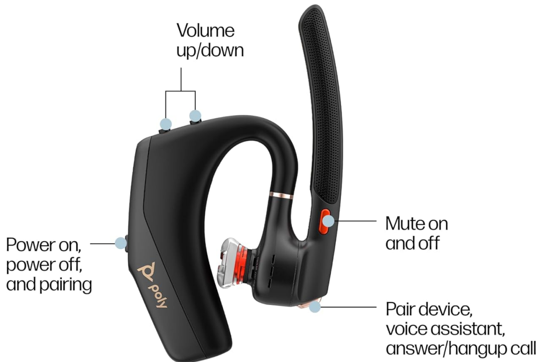
Image: A detailed diagram illustrating the intuitive button controls on the Poly Voyager Legend 50 UC headset, including volume, mute, power, and call management.
