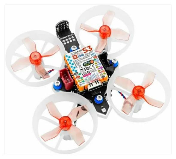
An overhead view of the M5Stamp Fly drone, showcasing its compact design, four propellers with protective guards, and the central M5StampS3 controller board. The board features various components and connectors, including a USB port.
