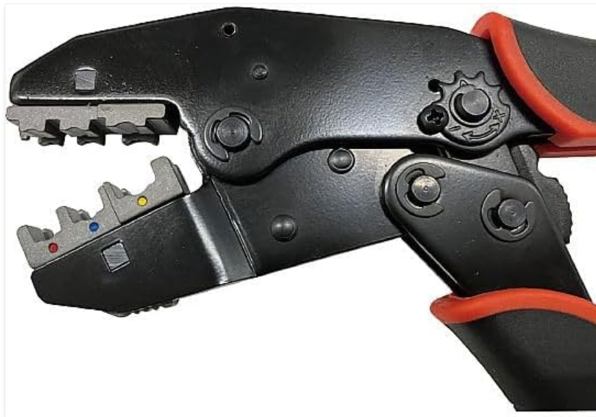
Image 3: A close-up view of the crimping pliers with one of the interchangeable dies securely inserted into the jaws, demonstrating proper setup.
