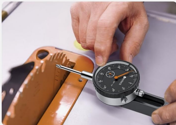
Check the Saw Blade Alignment and Run-out
