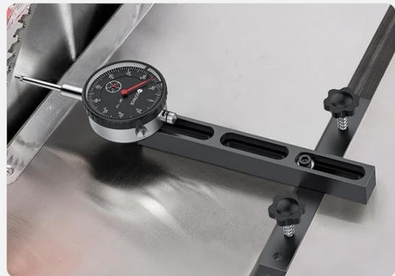
Check the Fence Straightness
