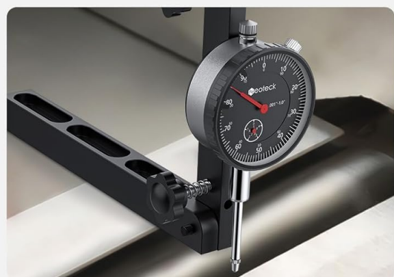
Check the Jointer Depth of Cut
