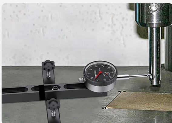
Check the Drill Chuck Run-out
