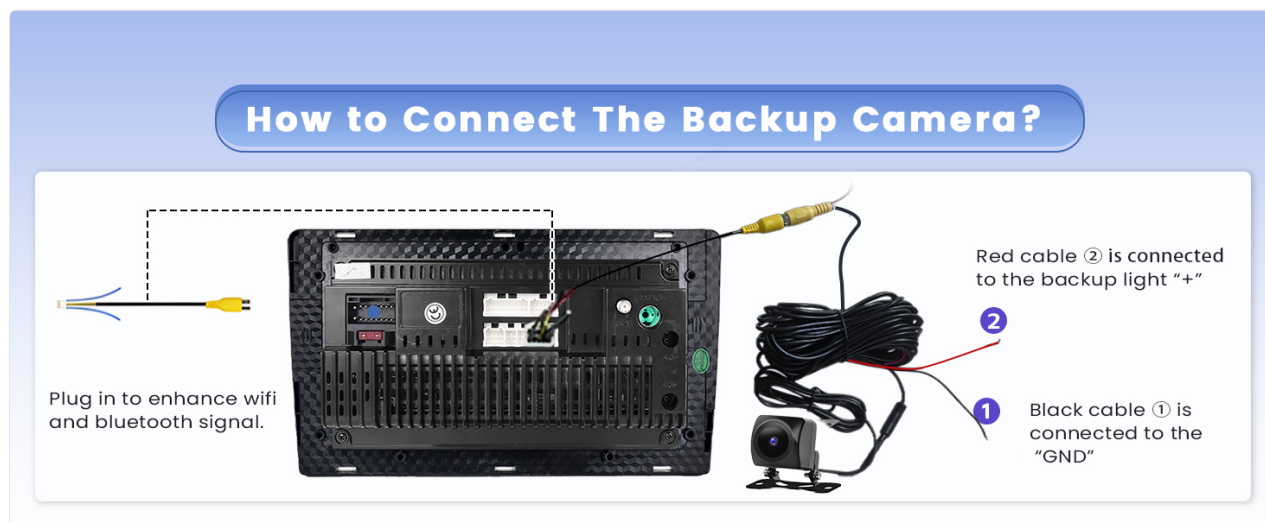
Image: Backup camera wiring diagram.
