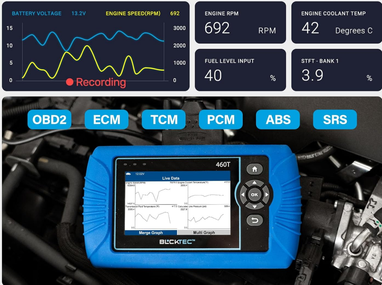
Figure 4.5: Real-Time OBD2 & OEM Live Data. Illustrates the dynamic live data visuals, including battery voltage, engine speed, engine RPM, engine coolant temperature, fuel level input, and short-term fuel trim, with options for OBD2, ECM, TCM, PCM, ABS, and SRS data.
