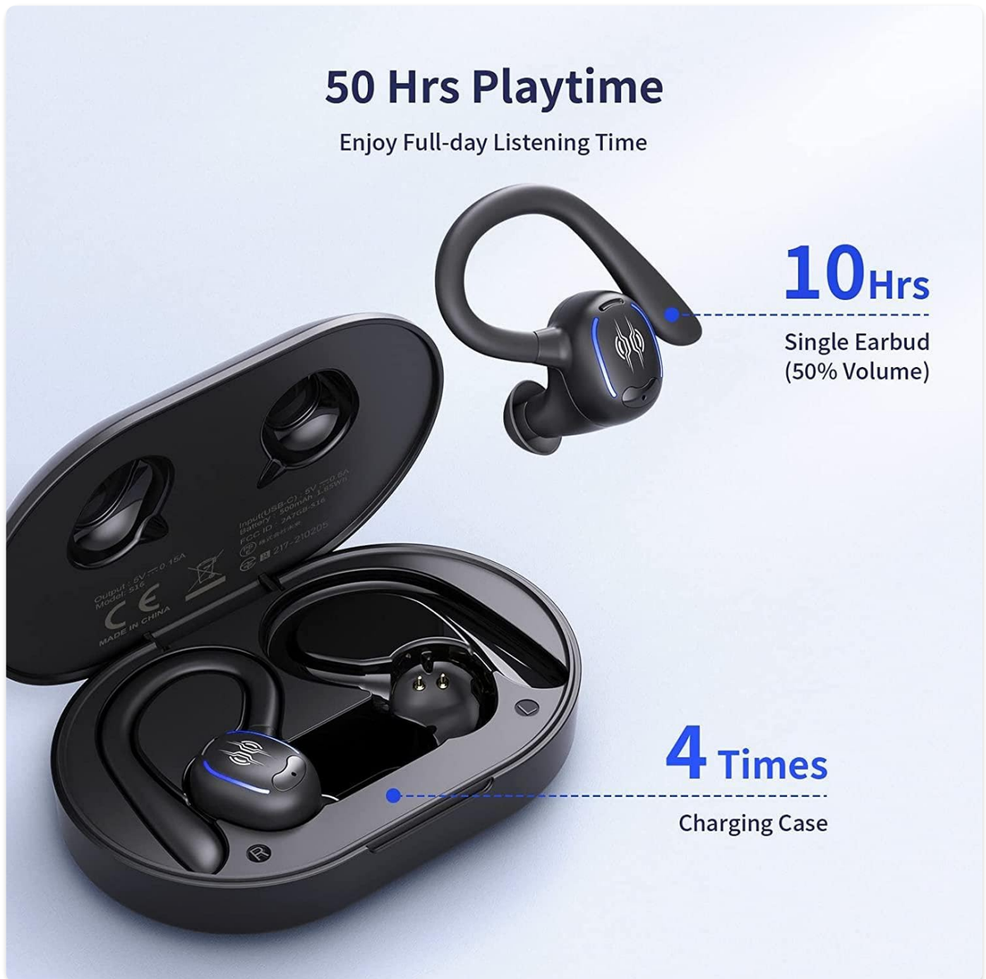
Image: An illustration demonstrating the extended playtime, showing 10 hours for a single earbud charge and 50 hours total with the charging case providing 4 additional charges.
