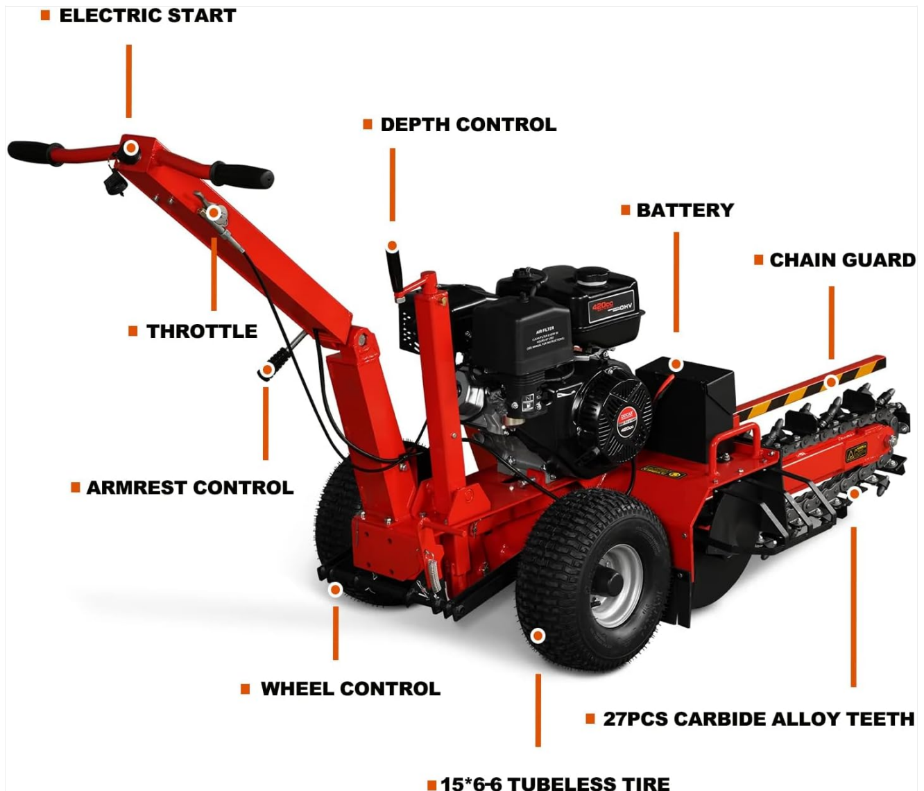
Figure 3.1: Key Components and Controls of the TCR1500 Trencher. Labels include Electric Start, Throttle, Armrest Control, Wheel Control, Depth Control, Battery, Chain Guard, 27pcs Carbide Alloy Teeth, and 15*6-6 Tubeless Tire.
