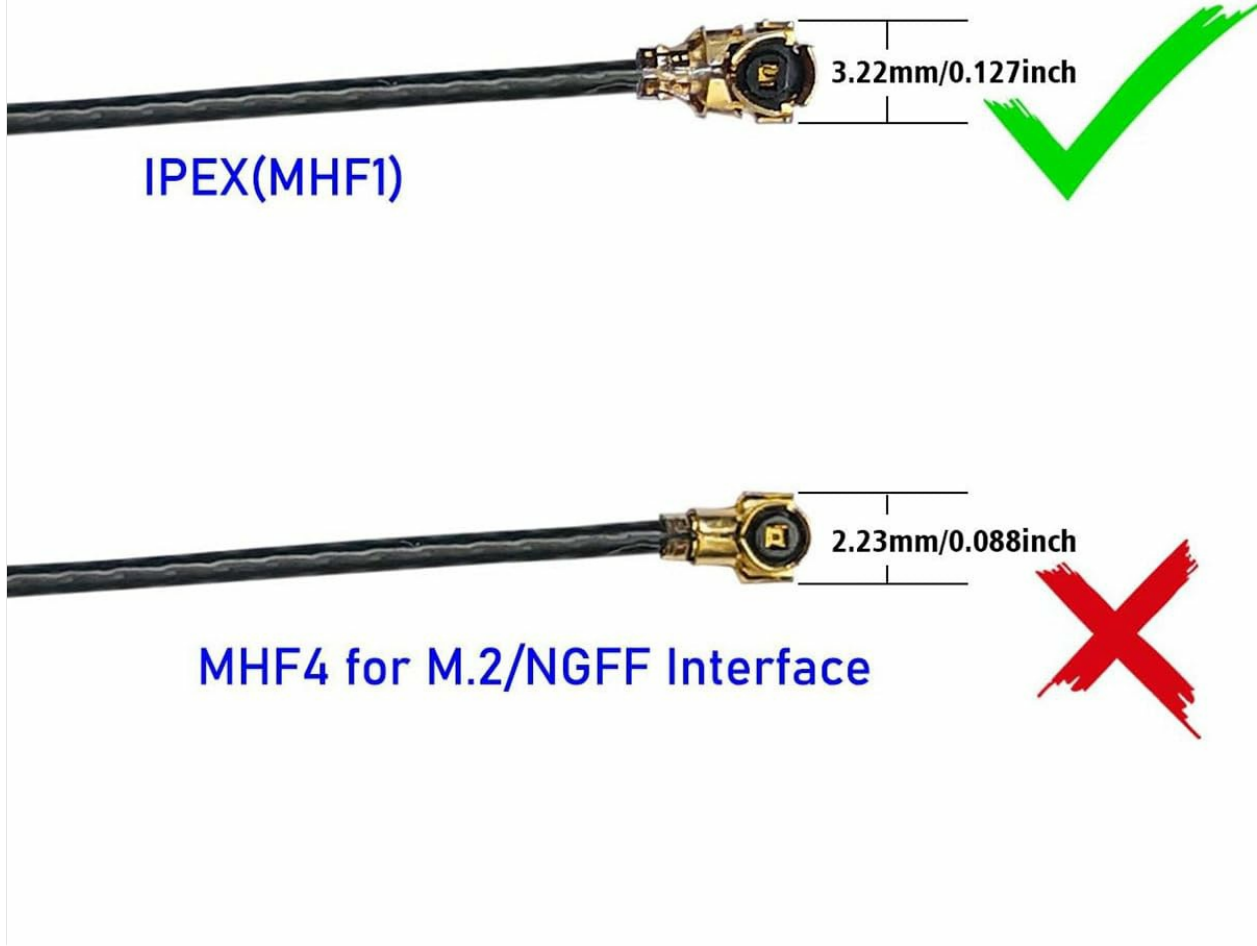
Image 3: Illustration of the correct IPEX(MHF1) antenna specification (3.22mm/0.127inch) for the Bluetooth antenna base, and an incorrect MHF4 antenna type.
