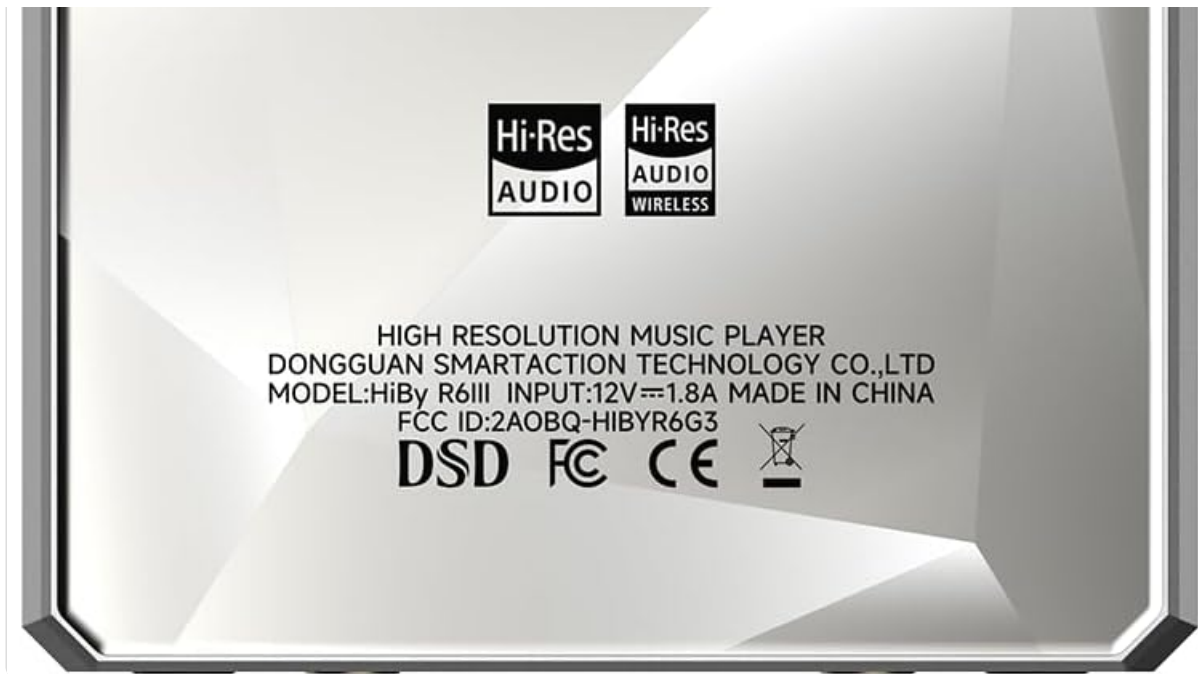
Figure 4.3: Back View. The back of the device features a diamond-cut glass backplate with the HiBy logo prominently displayed. "Hi-Res Audio" and "Hi-Res Audio Wireless" certifications are visible, along with regulatory information and the model number.
