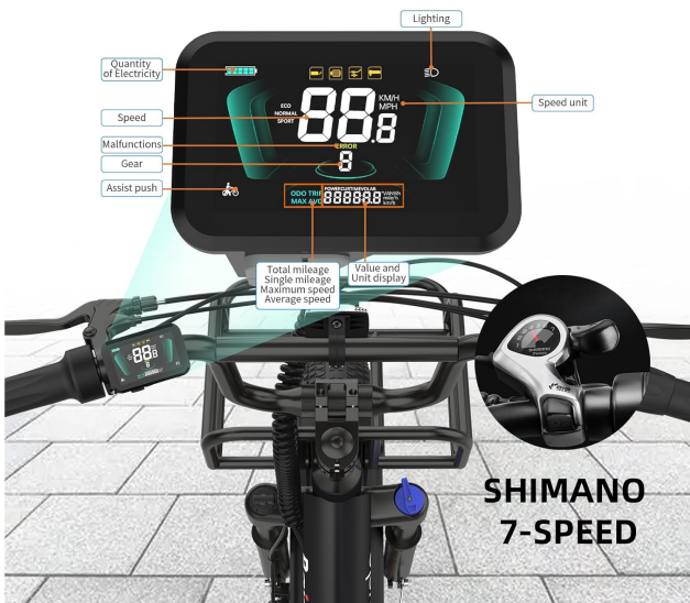
Figure 5: Color Smart LED Screen and Shimano 7-Speed
