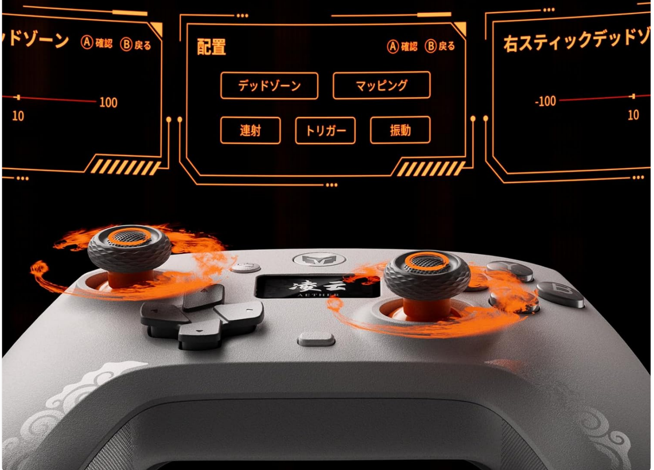
Figure 5: Core Algorithm Update for Deadzone Adjustment. This diagram illustrates the deadzone adjustment interface on the LCD, allowing precise control over joystick input, including 0 deadzone and negative deadzone settings.
