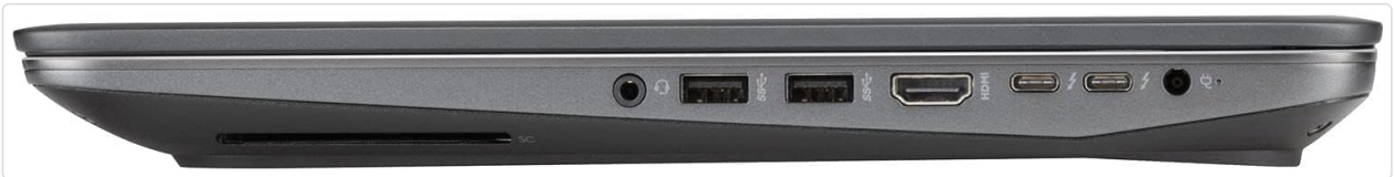
Image: Right side of the laptop, displaying the audio jack, two USB 3.0 ports, HDMI port, two Thunderbolt 3 ports, and power connector.
