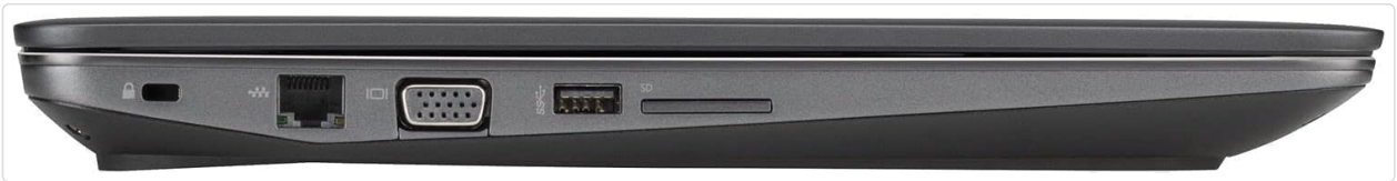
Image: Left side of the laptop, displaying the security lock slot, Ethernet port, VGA port, USB 3.0 port, and SD card reader.
