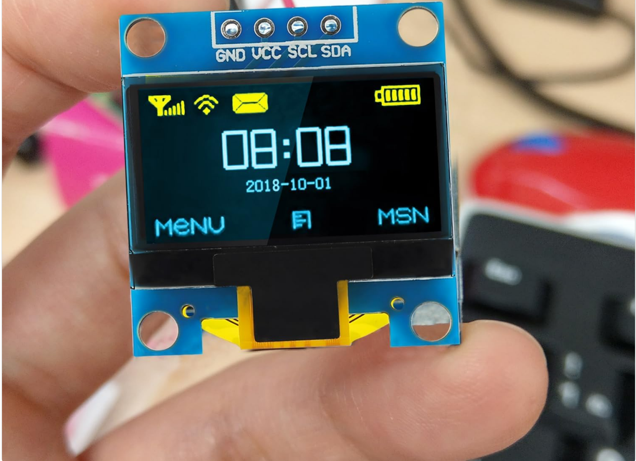
Image 2.2: The OLED module shown in a hand, illustrating its compact size and compatibility with common development platforms.
