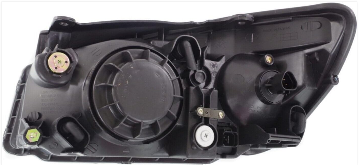
Figure 4.3: Rear view of the headlight assembly, showing the mounting points and electrical connectors for installation.
