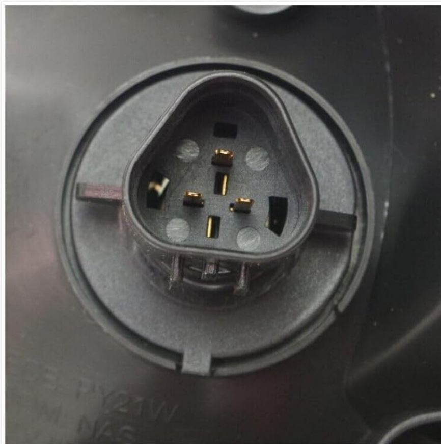
Figure 5.1: Example of a main electrical connector on the headlight assembly. Ensure it clicks into place.
