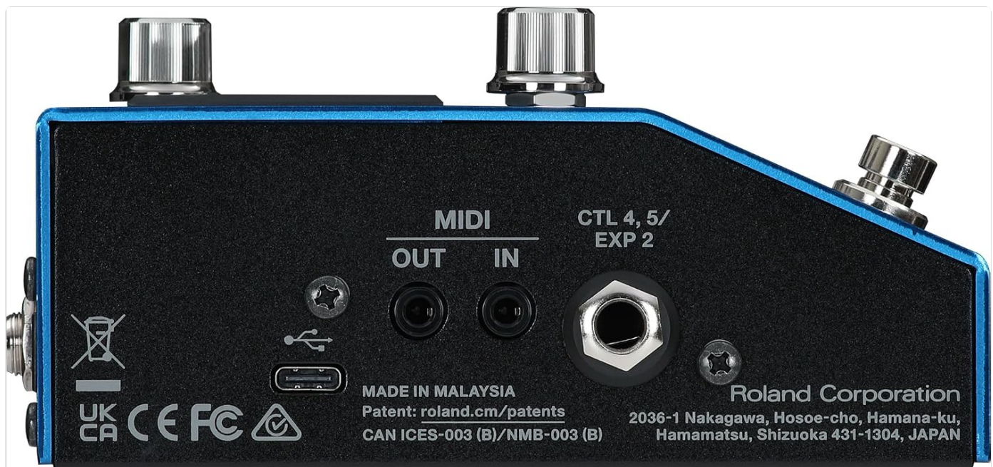
Image: The side panel of the VG-800, illustrating the MIDI IN/OUT, USB-C port, and additional control input jacks.
