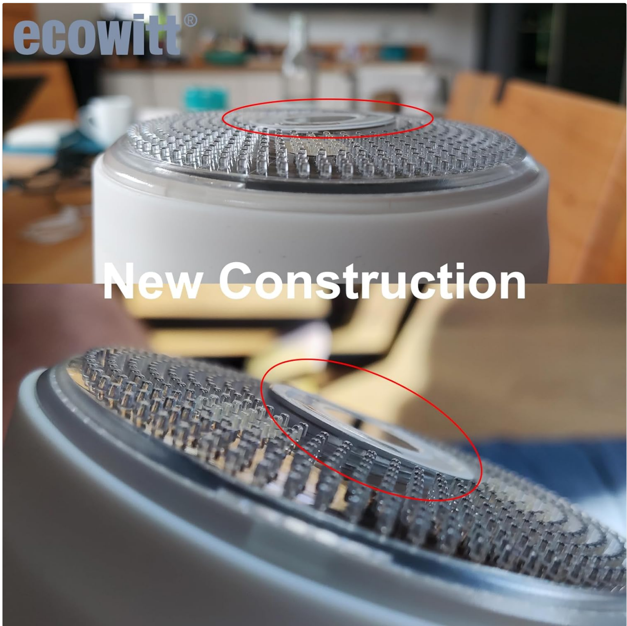
Figure 3.3: Detail of the WS90 haptic rain gauge, highlighting the new construction with an added slope to prevent water accumulation and improve rainfall measurement accuracy.
