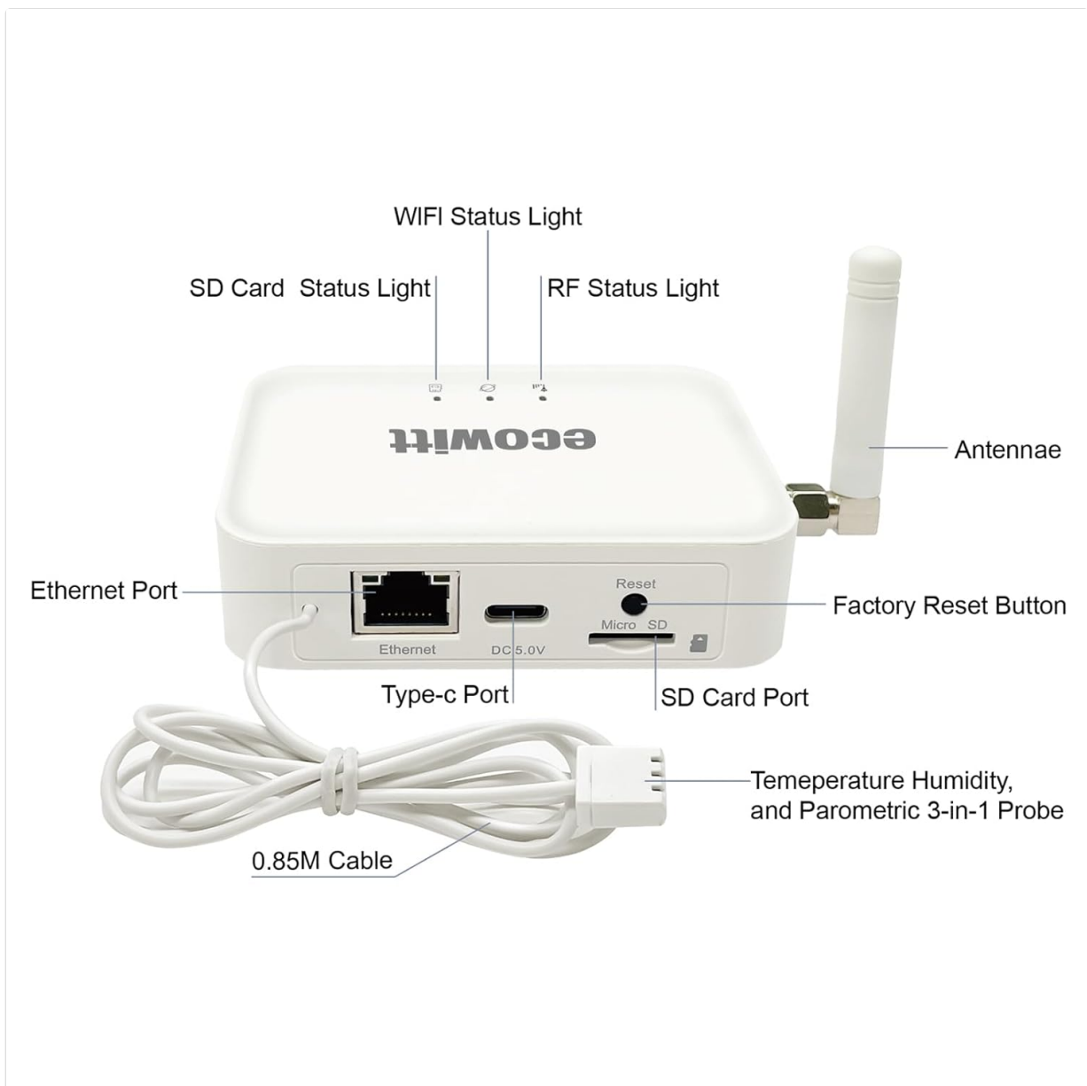
Figure 3.1: GW3000 Gateway with labeled components including Ethernet Port, Type-C Port, SD Card Port, Reset Button, Antennae, and status lights (WiFi, SD Card, RF).
