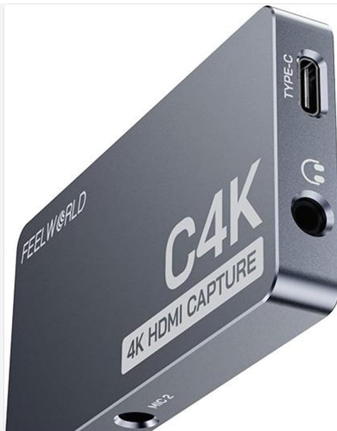
Image: Side view of the FEEWORLD C4K, highlighting the USB-C port for connection to a computer and the 3.5mm headphone jack.
