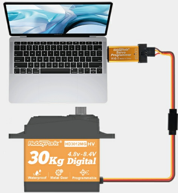
Image: Steps for programming the HobbyPark servo using a dedicated programmer and computer software.
