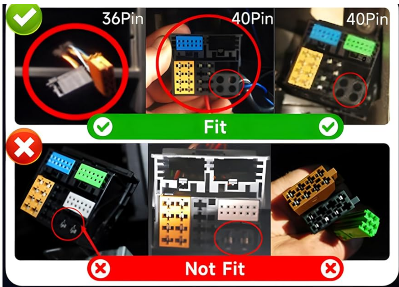
Figure 4.2: Correct and incorrect CANBUS plug connections.
