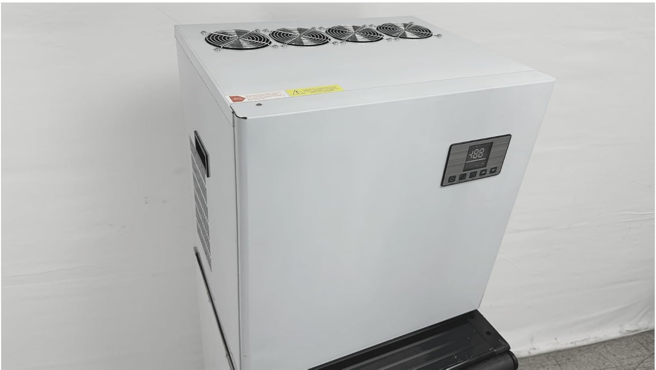
Figure 5.2: Top view of the ice maker, highlighting the ventilation fans for proper airflow.
