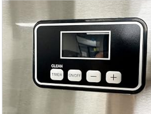
Figure 6.1: The digital control panel with various function buttons and display.
