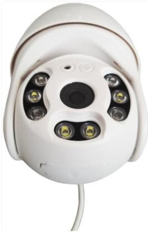
Figure 4.2: Close-up of the camera's front face. This view highlights the central camera lens, surrounded by various infrared and white light LEDs, and the microphone and speaker for two-way audio communication.
