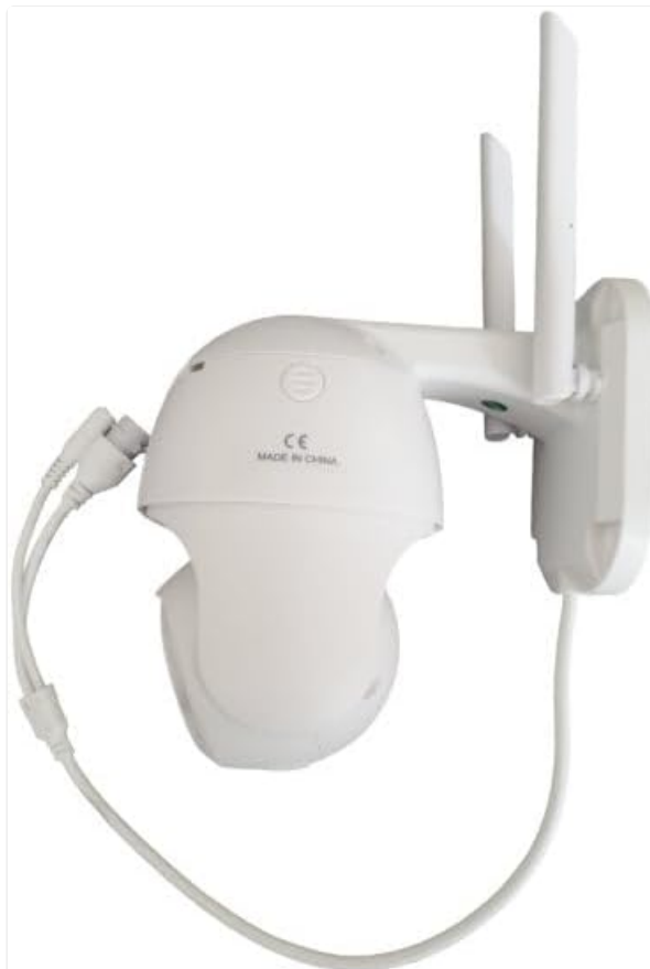
Figure 4.3: Side view of the camera mounted on its wall bracket. This image shows the camera's robust housing, the two Wi-Fi antennas, and the integrated power and network cables extending from the base for connection.
