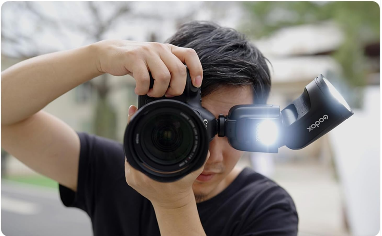
Figure 4.2: The GODOX V1 Pro V1Pro-F flash head demonstrating its horizontal swivel from 0° to 330° and vertical tilt from -7° to 120°. This range of motion allows for versatile light positioning and bounce flash applications.
