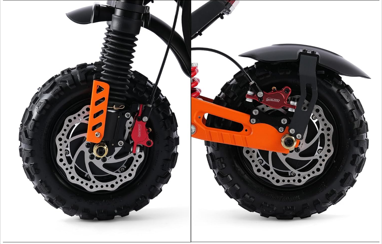
Figure 6.3: Front and Rear Hydraulic Disc Brakes.
