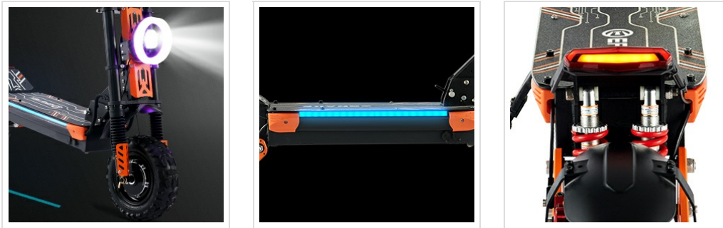
Figure 5.2: Front Headlight, Side Ambient Lights, and Rear Brake Light.
