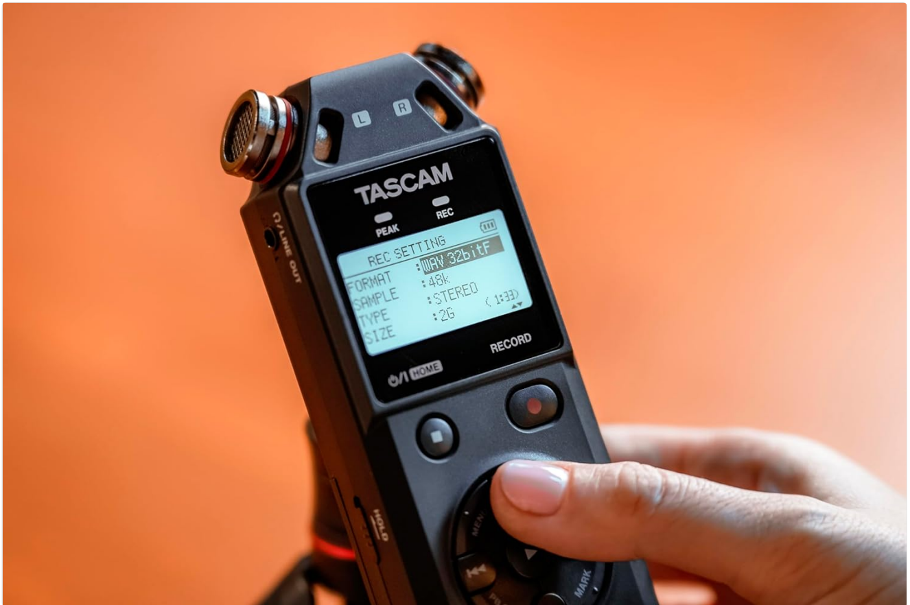
Figure 5: A hand interacting with the TASCAM DR-05XP, showing the LCD screen displaying recording settings such as format, sample rate, and type.
