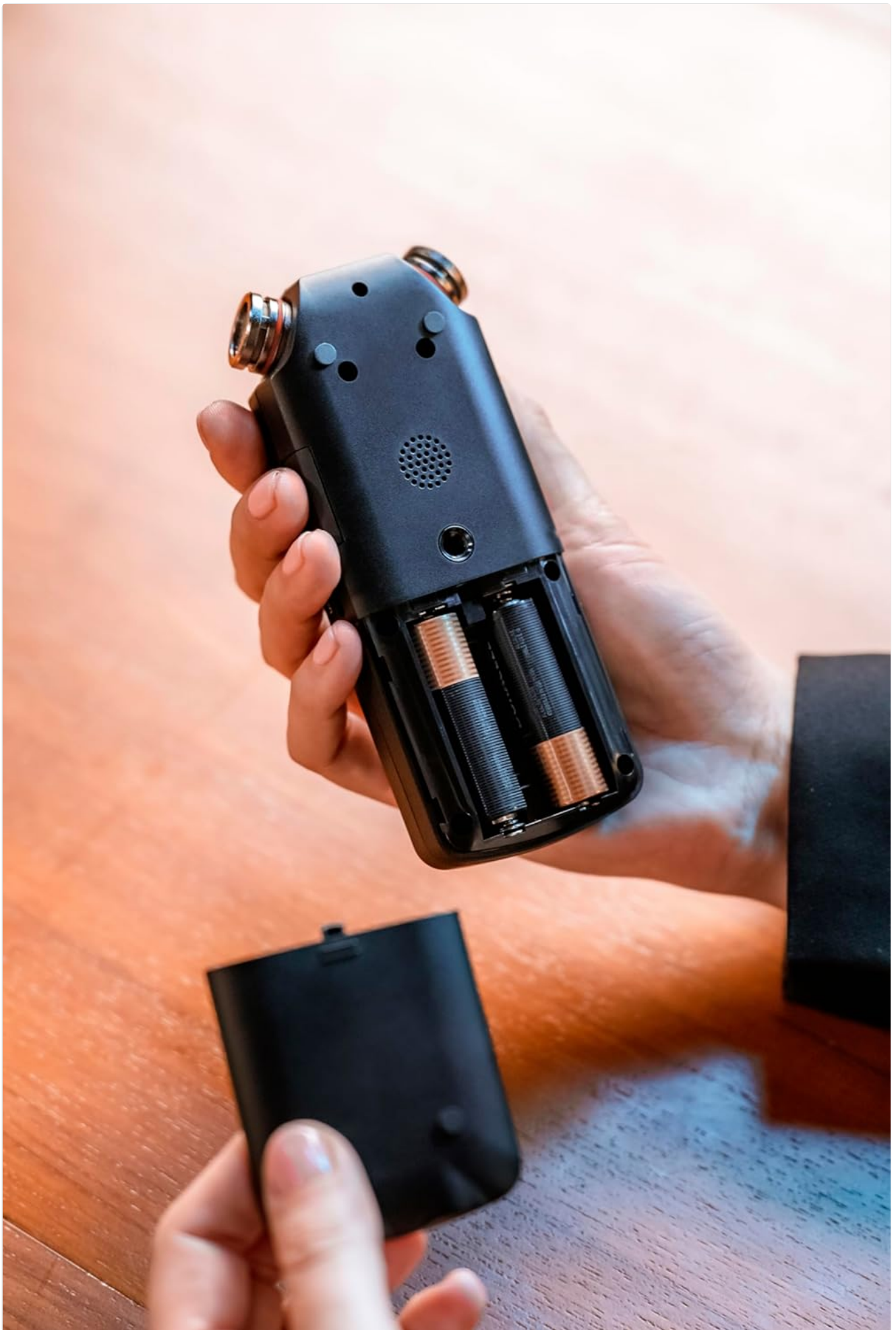
Figure 2: A hand inserting two AA batteries into the battery compartment located on the back of the TASCAM DR-05XP recorder.
