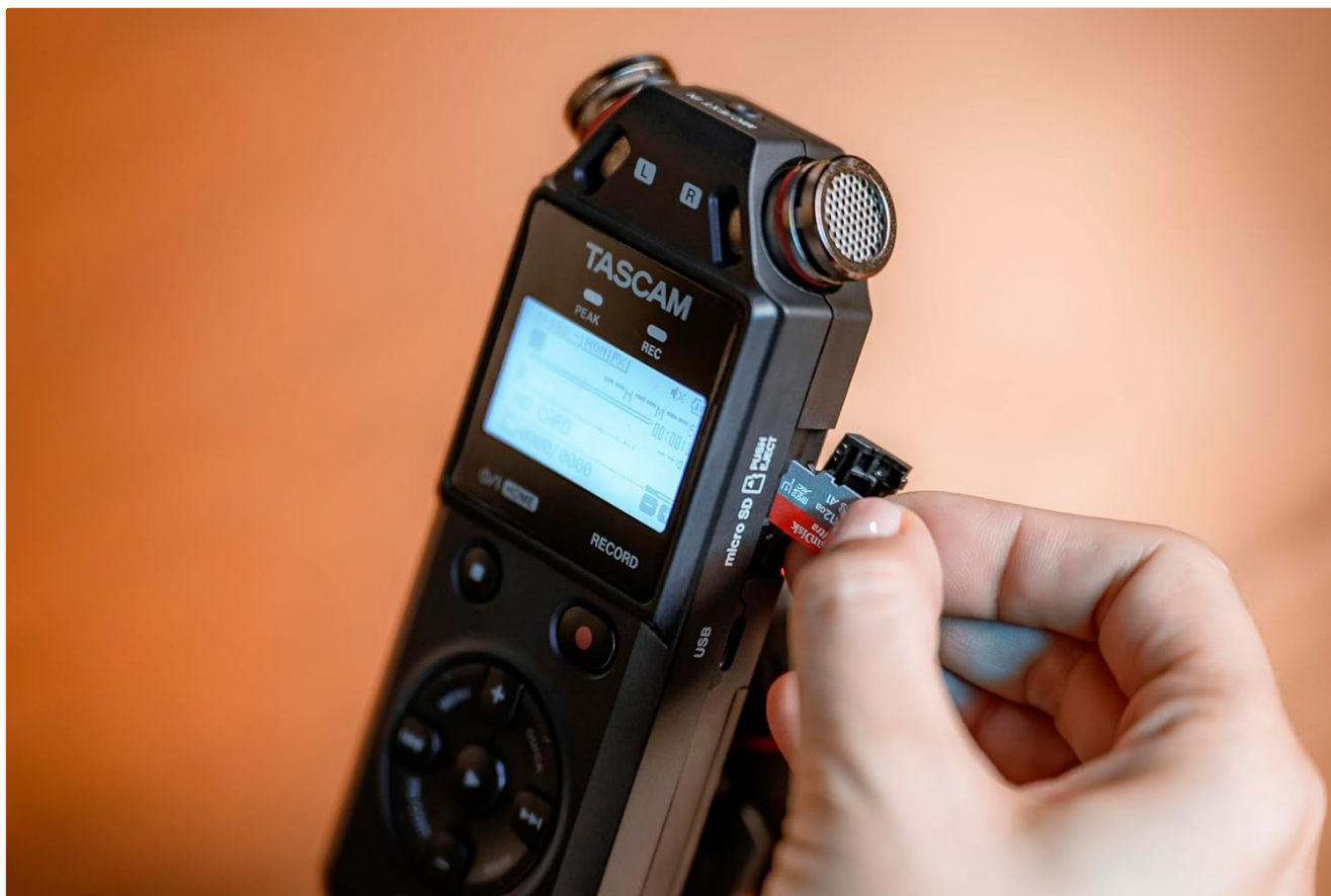
Figure 3: A hand inserting a Micro SD card into the dedicated slot on the side of the TASCAM DR-05XP recorder.
