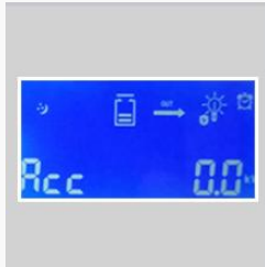
Figure 9: Display showing accumulated discharge.
