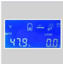
Figure 8: Display showing battery voltage and load current.
