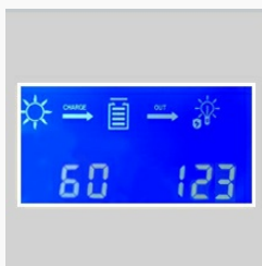
Figure 6: Display showing cumulative power generation.
