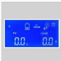
Figure 7: Display showing PV voltage and load power.
