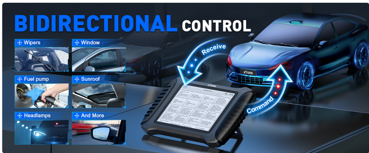
Image 4.2: Illustration of bi-directional control functionality, sending commands to vehicle components.
