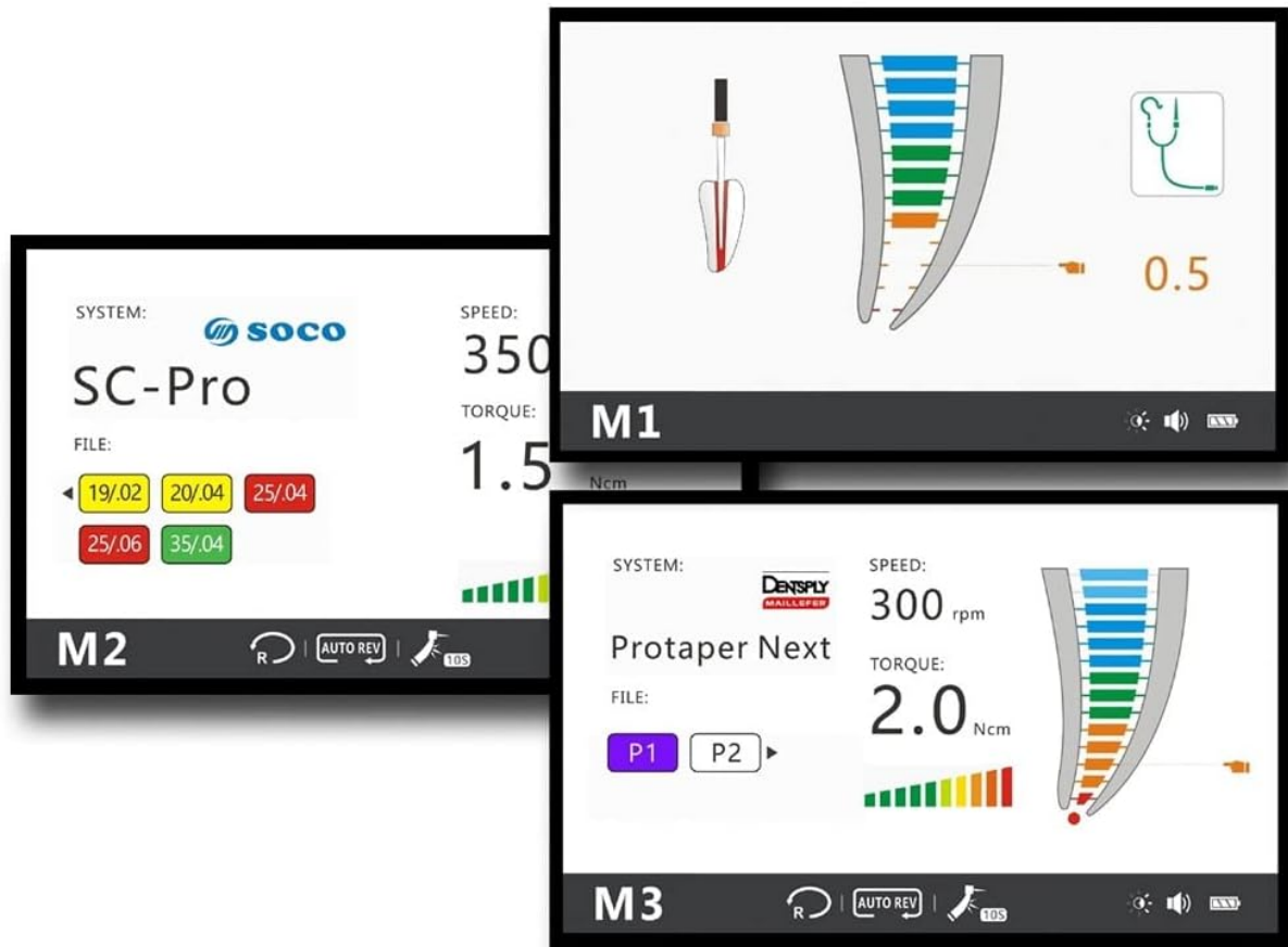
Figure 6.1: Three Work Modes (M1, M2, M3). This image illustrates the different display configurations for each working mode, showing variations in speed, torque, and file system selection.
