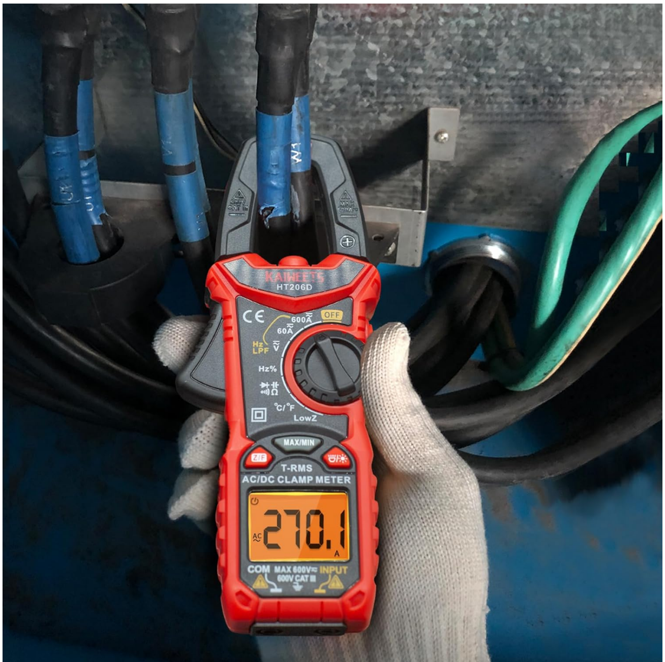
Image 5.1.1: KAIWEETS HT206D Digital Clamp Meter measuring current.
