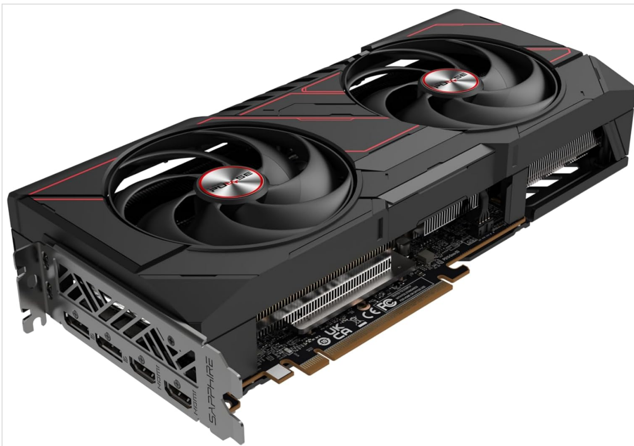
Image 3.1: Display output ports on the graphics card.
