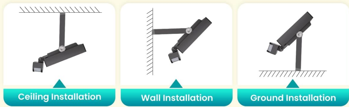
Image 5.1: Diagram showing the dimensions of the floodlight, the 180° adjustable bracket, and various installation methods including ceiling, wall, and ground mounting.
