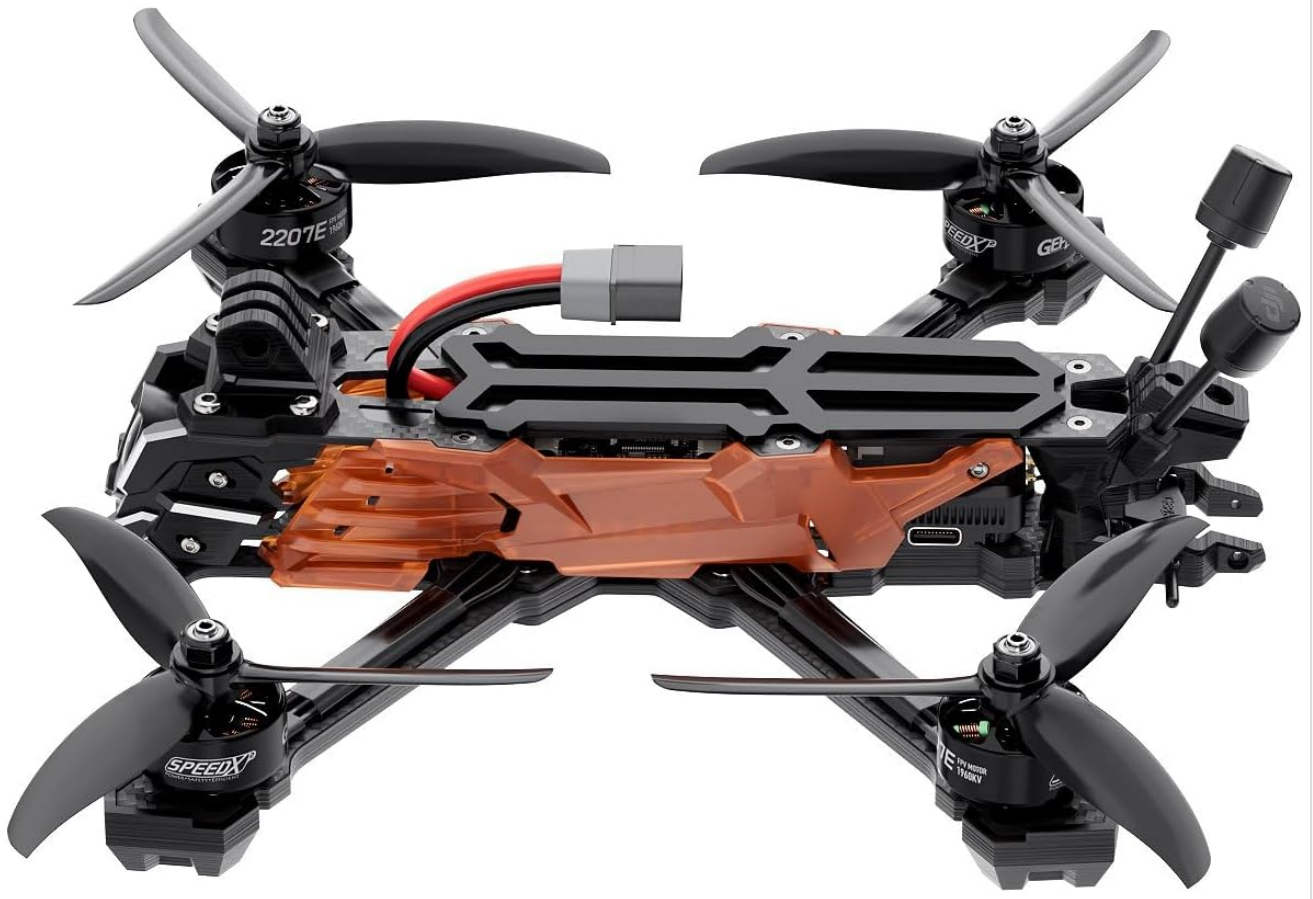
Figure 2: Top-down view of the GEPRC Vapor-X5 HD O4 Pro FPV Drone, highlighting the central electronics bay and battery strap area.
