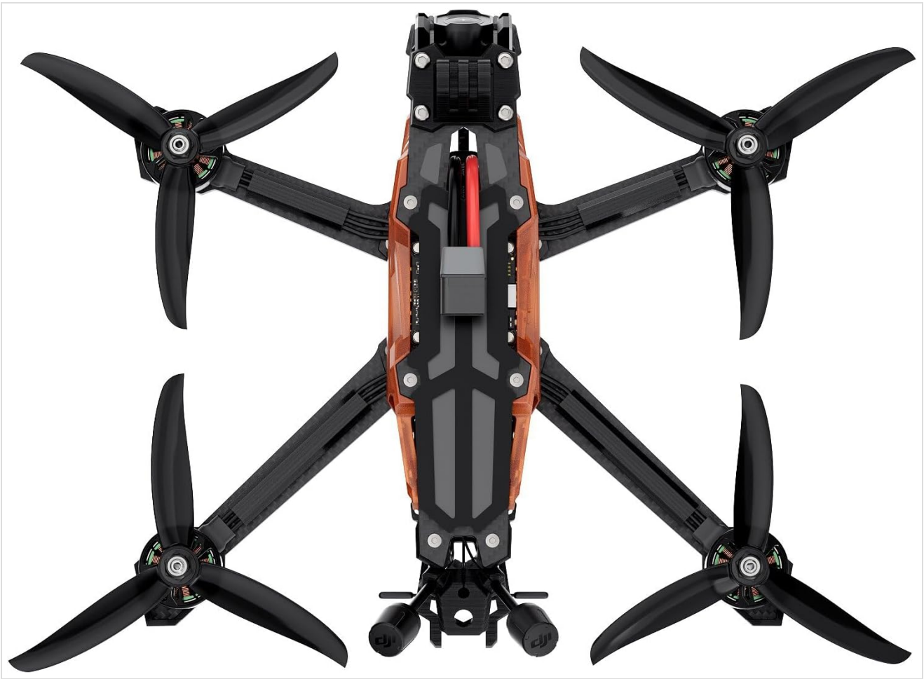
Figure 6: Bottom view of the drone. This image displays the motor mounts and the propeller attachment points.
