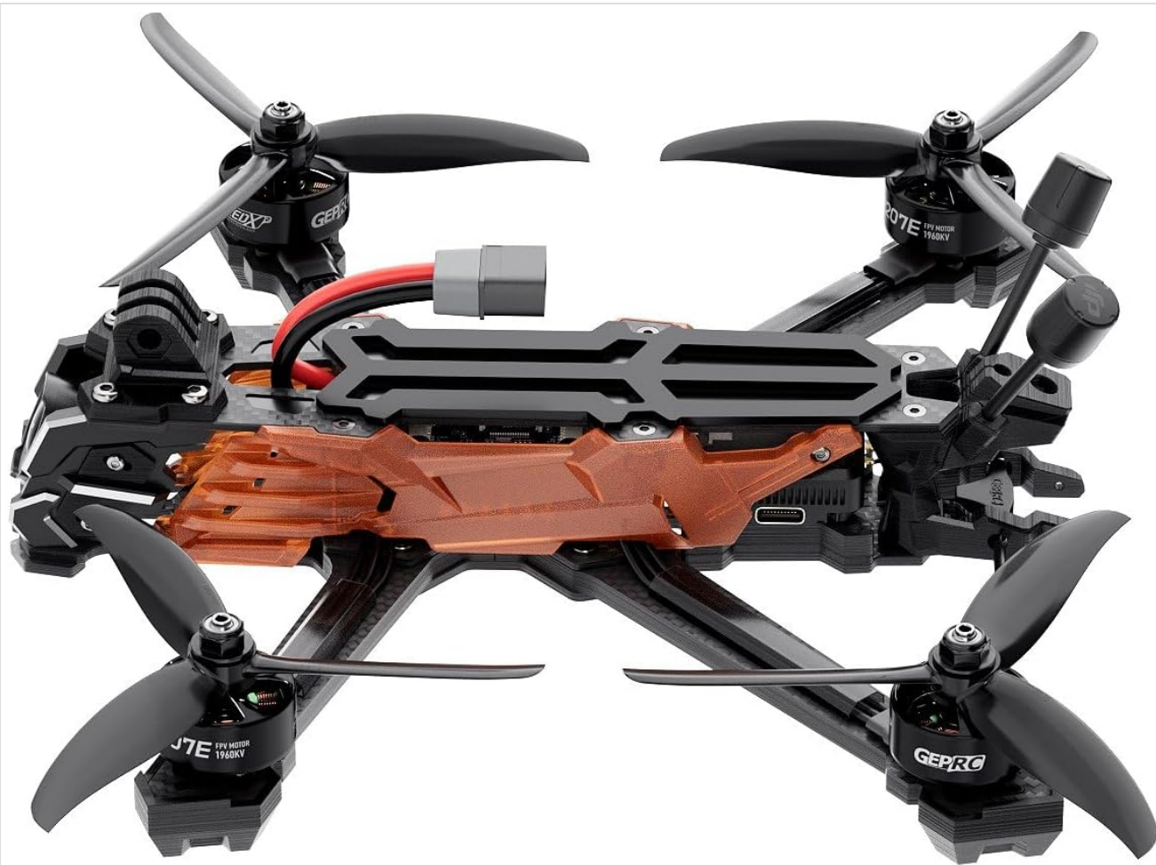
Figure 2: Top view of the drone. This perspective illustrates the central frame, battery strap area, and the arrangement of the four propellers.
