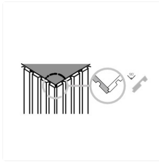
Image: Diagram illustrating the method for installing panels around a 90-degree corner, highlighting the interlocking profile.
