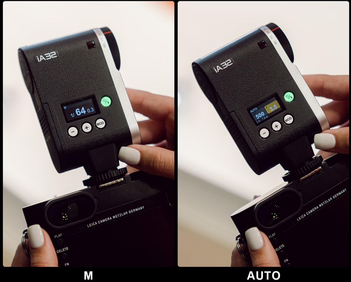
Image: The LCD panel of the Godox iA32 flash, illustrating the display in both Manual (M) mode with power level setting and Auto mode with recommended shooting distance.
