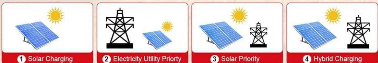
Figure 5: Visual representation of the four user-configurable charging modes for the inverter's battery system.
