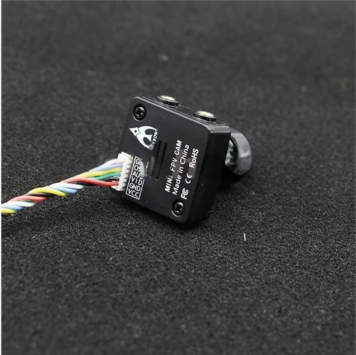
Figure 3.1: Example of an FPV camera connected using a multi-pin cable. Note the pinout labels on the camera.
