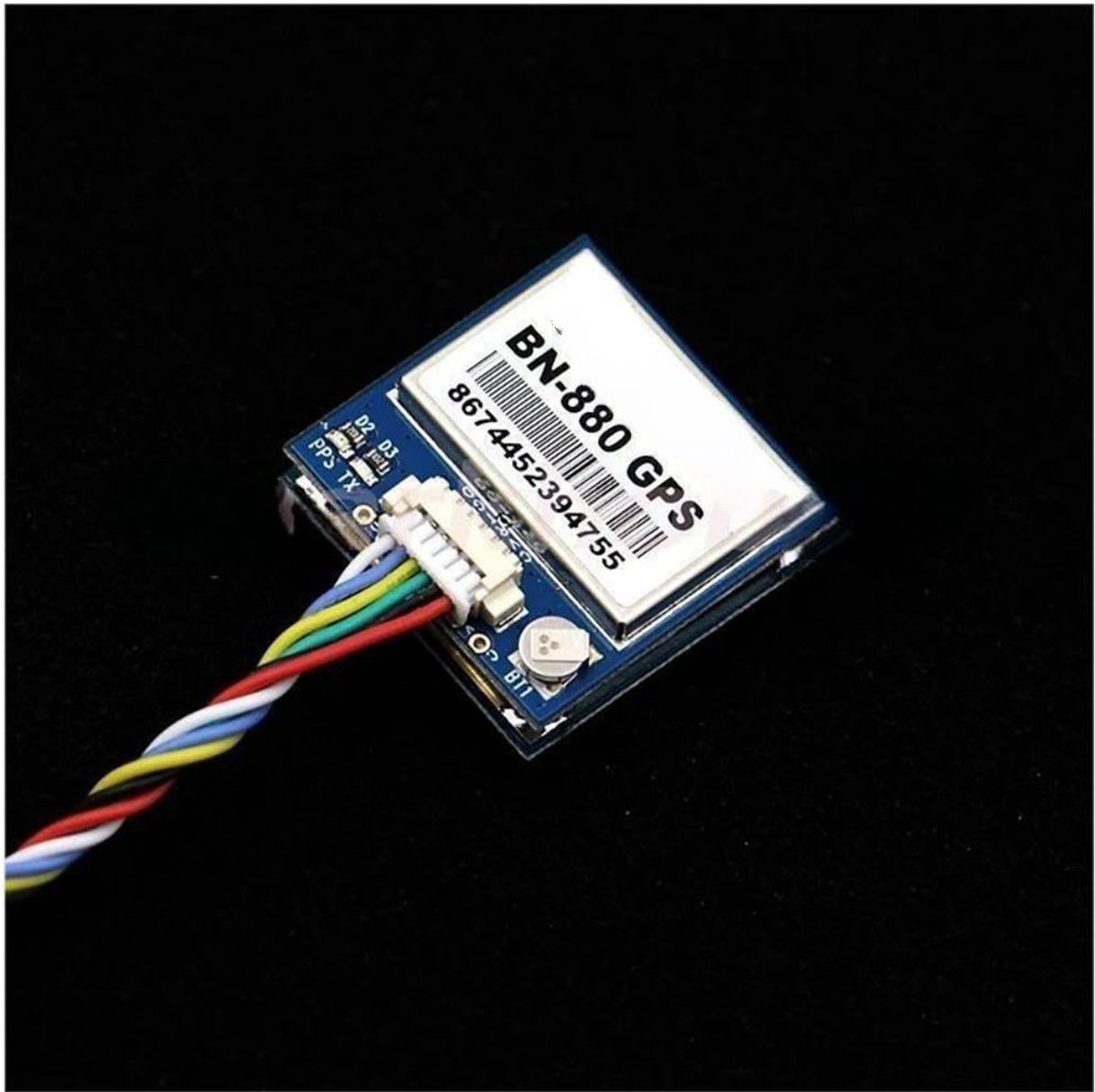
Figure 3.2: Example of a BN-880 GPS module connected with a multi-pin cable, showing the connection to the module's port.
