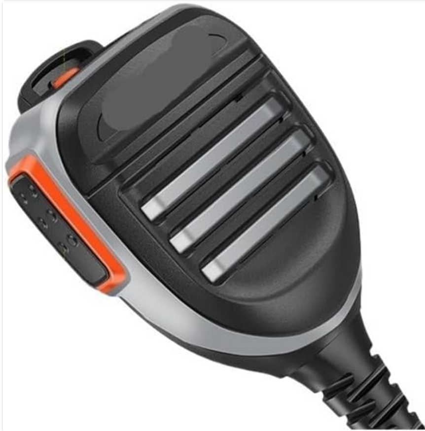
Figure 3: Side view illustrating the PTT button and speaker grille.
