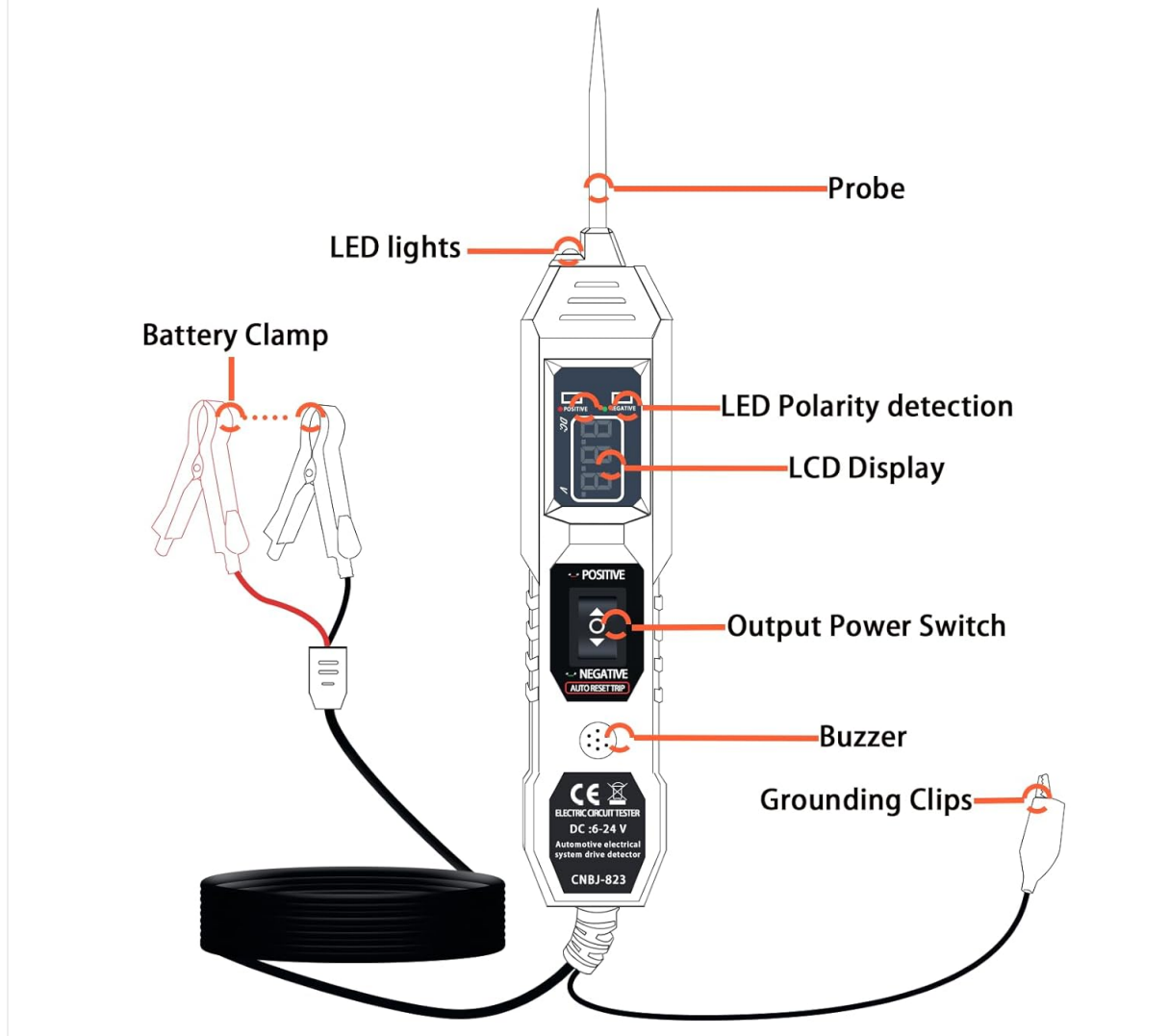
Figure 2: Key components of the Lqito Car Circuit Tester, including the probe, LED lights, battery clamp, LED polarity detection, LCD display, output power switch, buzzer, and grounding clips.
