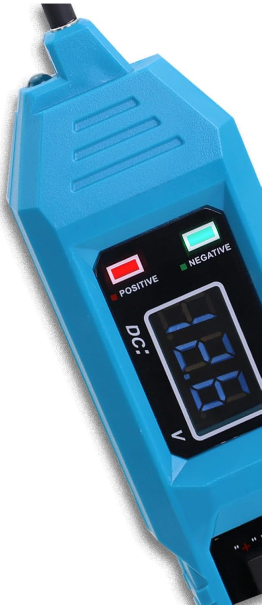
Figure 4: The tester's display clearly indicates voltage and polarity with red (positive) and green (negative) LEDs.
