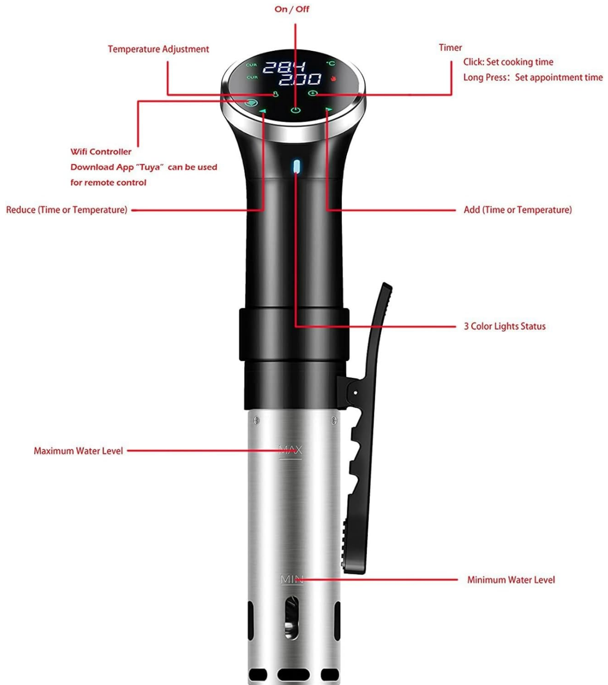
Image 3.1: Detailed view of the Sous Vide Cooker's control panel and main components, including buttons for On/Off, Temperature Adjustment, Timer, Wifi Controller, and water level indicators (MAX/MIN).
