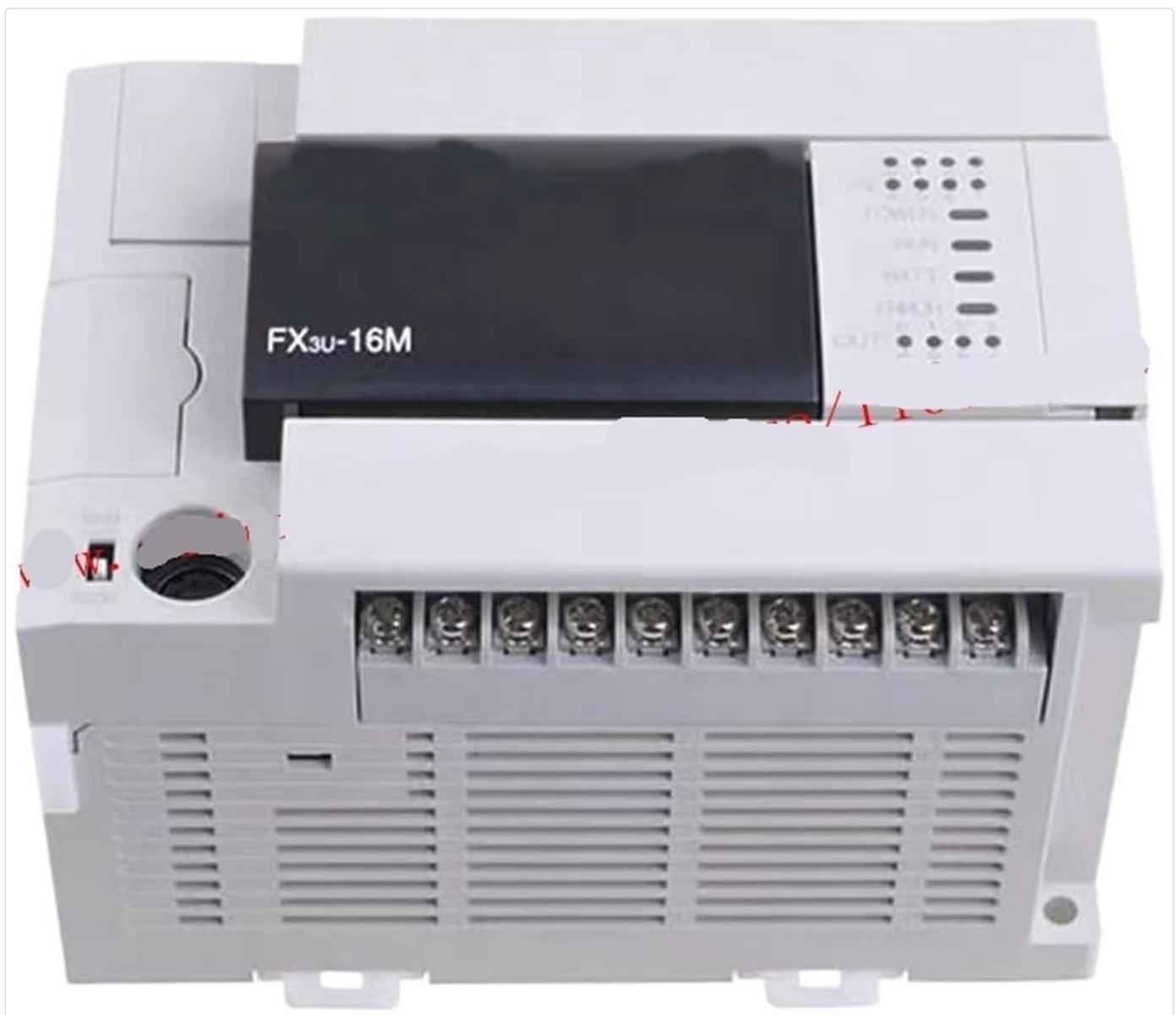
Figure 3.1: Front view of the NHJLFKSA FX3U series PLC module, showing power indicators, terminal blocks for inputs and outputs, and the model designation. This view highlights the main operational interface.
