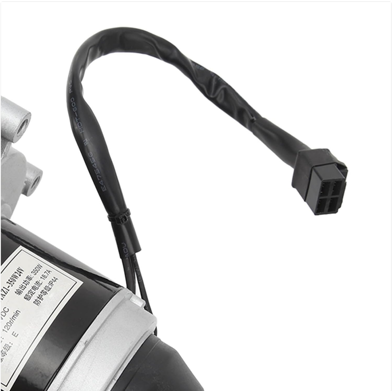
Figure 5.1: Close-up of the motor's electrical connector, which should be securely connected to the wheelchair's control system.
