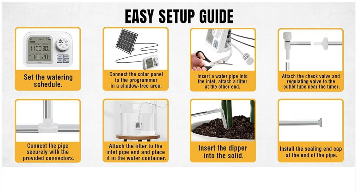
Figure 3: Easy setup guide illustrating the connection process for the irrigation kit.
