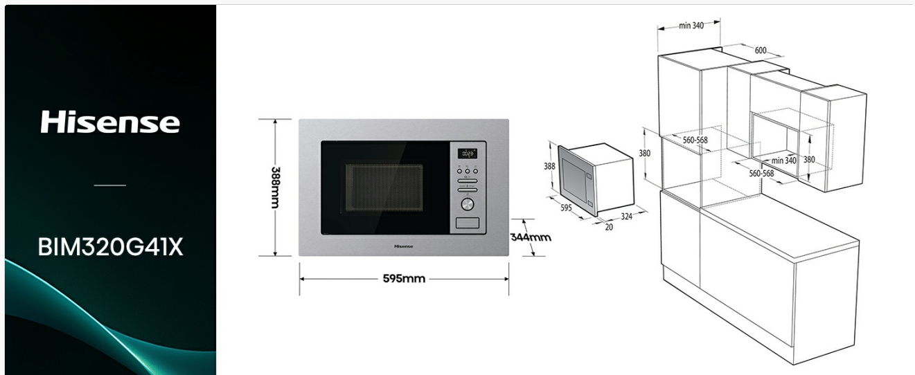
Image: Technical drawing showing the dimensions of the Hisense BIM320G41X microwave and the recommended cabinet opening for built-in installation.
