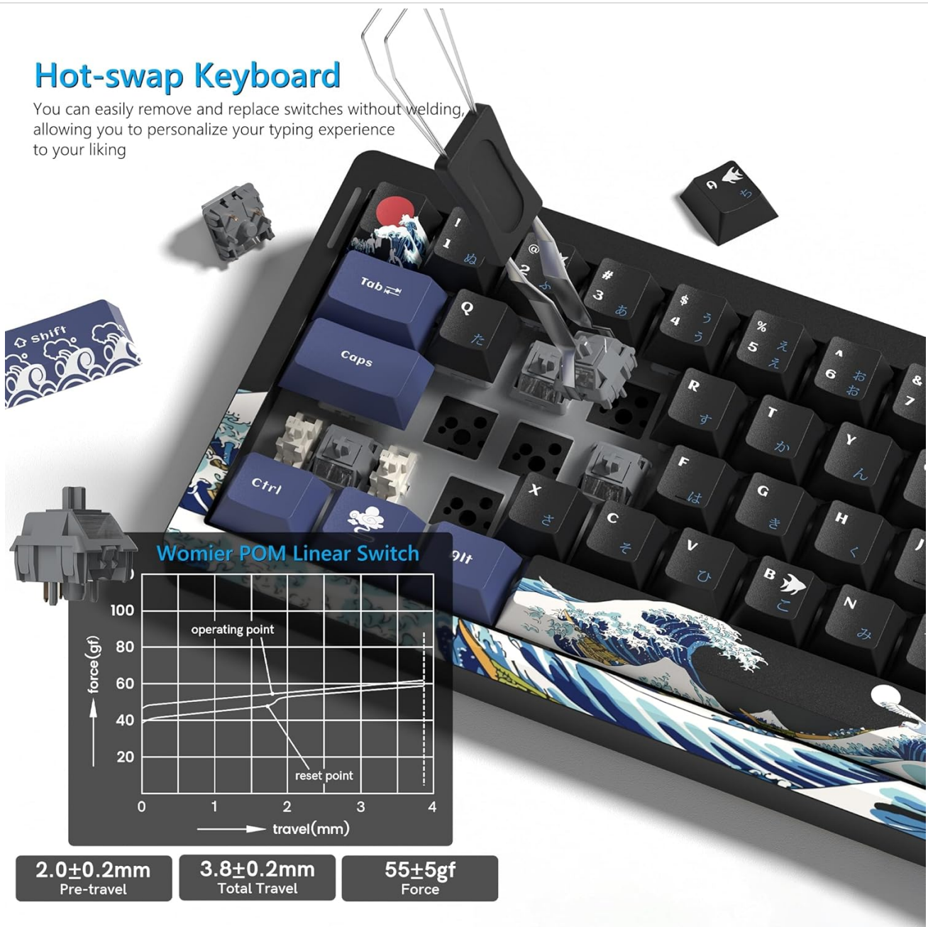
Image 6: Visual guide demonstrating the process of hot-swapping mechanical switches on the Womier Q61-Kanagawa keyboard.
