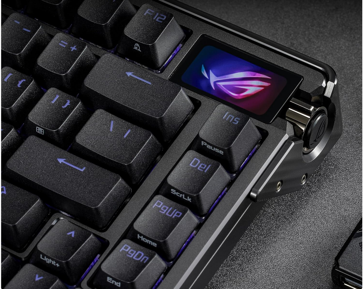
Image 3.4: The full-color OLED touchscreen and adjacent three-way control knob, used for displaying information and adjusting settings.
